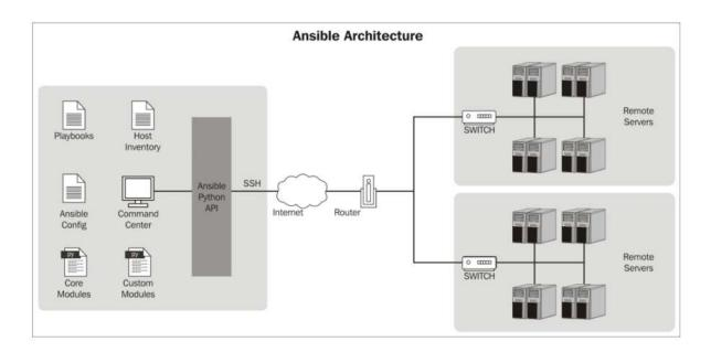
The host inventory file determines the target machines where these **plays** will be executed. The Ansible configuration file can be customized to reflect the settings in your environment. The remote servers should have Python installed along with a library named simplejson in case you are using Python Version 2.5 or an earlier version.
